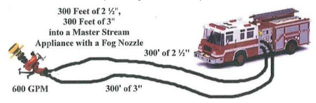
Divide the total GPM by the number of hose lines (600 GPM divided by 2 = 300 GPM), using the conversion factor for 3" hose, compute the equivalent flow through 2  $\frac{1}{2}$ " hose (2/3 x 300 GPM = 200), then compute the friction loss rate for 200 GPM and 300 GPM.
