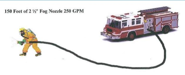
The firefighter is ordered to pull the standard 150' 2 ½" pre-connect. Since a specific GPM has not been asked for, use 250 GPM (predetermined GPM for 2 1/2" fog nozzle).
