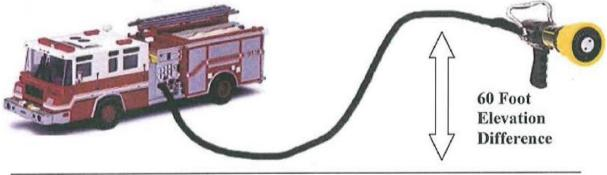
The firefighter is ordered to pull 600' of 2 ½" working line un an incline. The company officer requests 200 GMP from a standard fog nozzle. To set this problem up, identify what information you will need to solve the problem. In this case, you will solve for Pump Pressure (PP)
