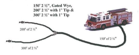
PP=NP + FLR x L + FLR x L PP=50 + \_\_\_\_ x 1.5 + \_\_\_\_ x 2.5 (200' & 300' Averaged)
